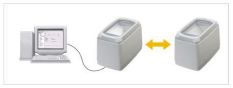
You can control the QK20/21 models by sending commands from a host device such as a PC or POS register.
