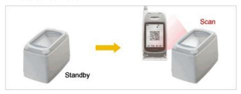
The code is automatically read as soon as it is detected within the reading field of vision.
