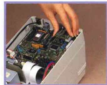
Option 2 :Interface board (RS-422A,20mA current loop:user installable)
